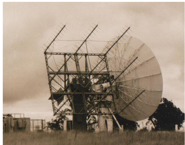
Cooby Creek tracking station phased yagi array with satellite dish in the background. Photo Courtesy of HullWarren
